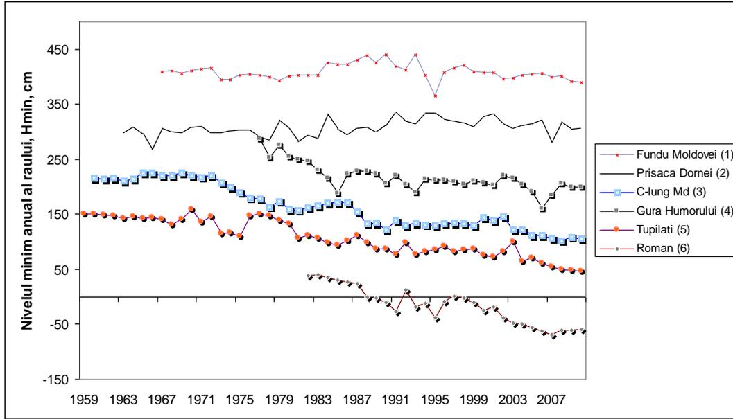
Fig. 13 Vertical dynamics of the channel bed level of Moldova river estimated based on the minimum annual level in 6 cross sections along the river
