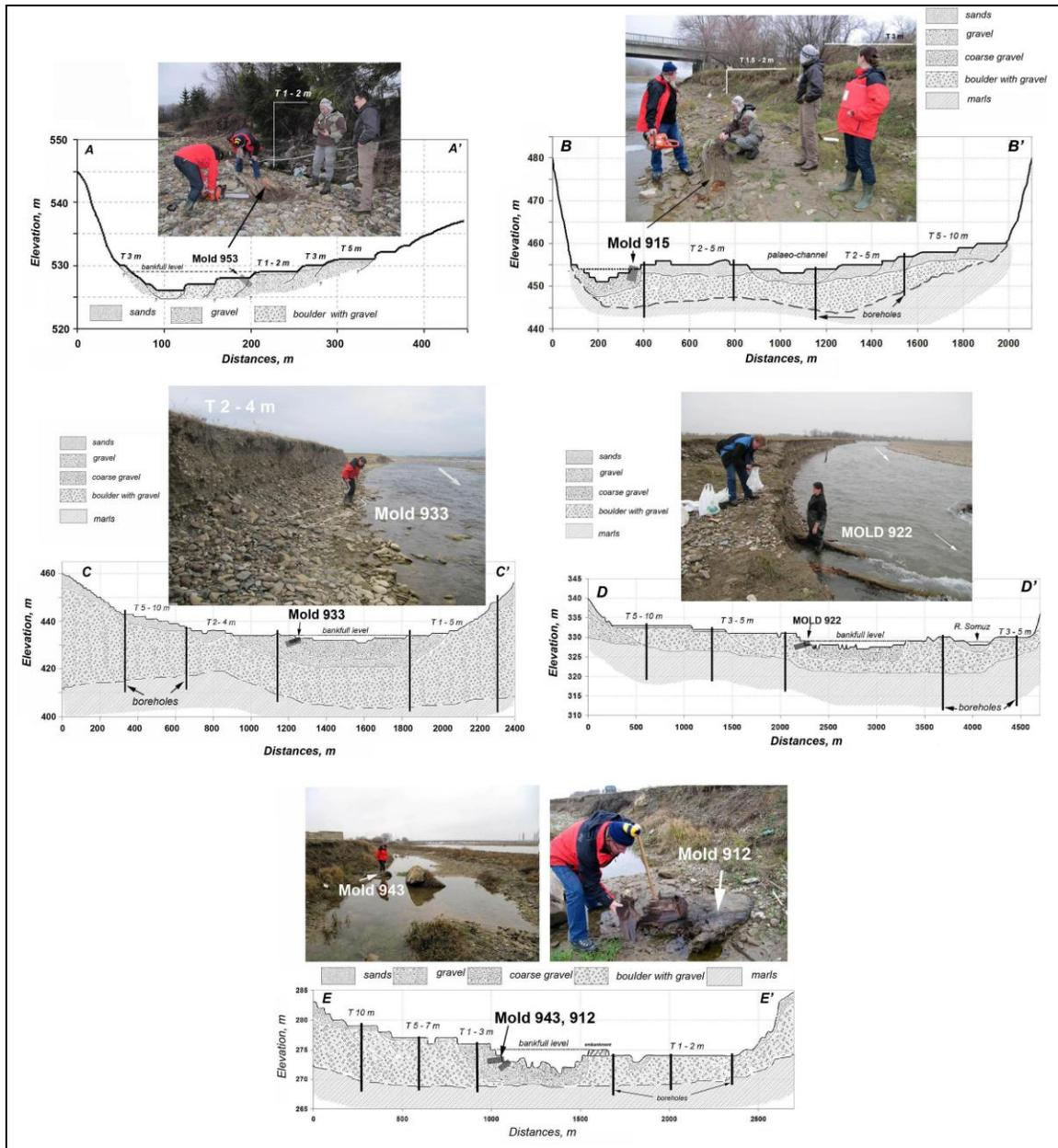
Fig. 14 Geomorphological profiles along Moldova valley: Moldid (Mold 953); Gura Humorului (Mold 915); Slatina (Mold 933); Vadu Moldovei (Mold 922); Timișești (Mold 943,912) (Chiriloaei et al., 2012).
