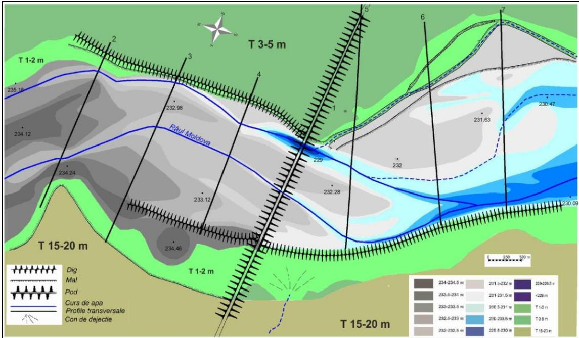
Fig. 5 Geomorphological sketch of Moldova river bed in Tupilați gauging station
